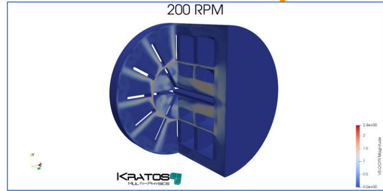
Relative Temporal Average Velocity for Various RPMs (Mesh Velocity Subtracted).
